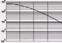
電容器 (絕緣電阻) 的變化圖示 Insulation resistance as a function of temperature.
